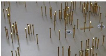
Spring-loaded “pogo pins” are the industry-standard interface for in-circuit test fixtures. Microlynx uses high quality precision pins that are rated to over a million cycles. Tips are field replaceable in the event of wear or damage.
