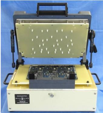
Improve the quality of your electronic products through In-circuit Electrical Testing (ICT). At even moderate production volumes, a Microlynx test jig will quickly pay for itself and start saving you money by reducing the test time and reducing waste and warranty costs.
